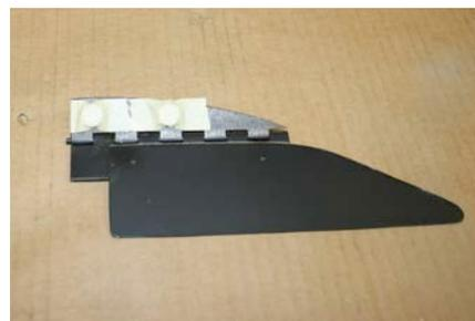
4. Push the screws through the tape and washers from the firebox side to the door frame side.
