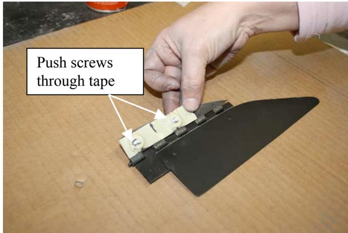
5. Locate the mounting holes inside the firebox. Hold the smoke deflector up to the holes and start the screws by hand. Be sure the flat hinge side is facing you.
