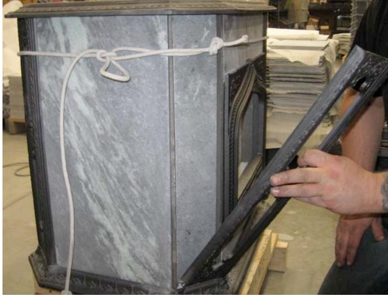
9. Remove the corner stone. Tighten the rope.
