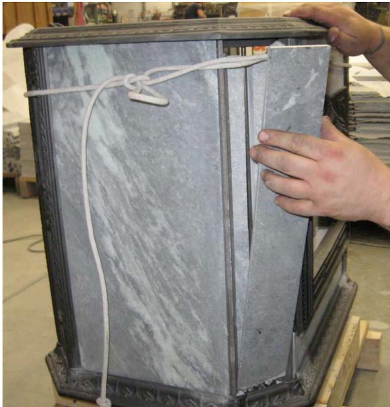
10. Apply a generous amount of furnace cement to the top, beveled edge of the new stone so that there is about a 1/2" of cement where the bevel meets the inside edge of the top frame. This will ensure a proper seal in this area.
