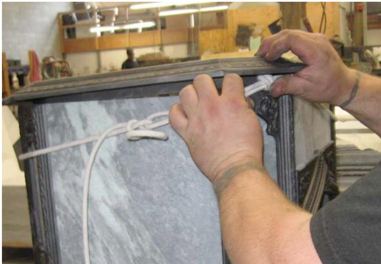
13. Lower the top frame back down making sure that it securely overlaps the top edge of the corner cast. Tap gently with the rubber mallet if necessary.
