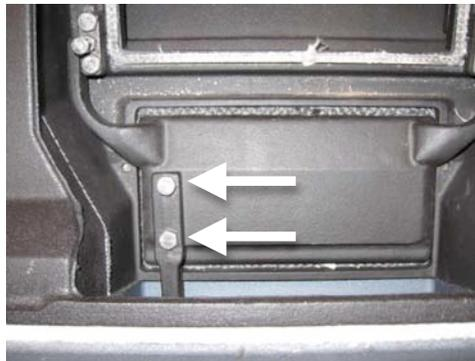
5. Completely remove the front bolt from each of the bypass retainers, and loosen the rear bolt using a  $\frac{1}{2}$ " wrench. It may be necessary to remove the center  $\frac{1}{4}$ "-20 x1" bolts, (loosen lock nuts first) using  $\frac{7}{16}$ " socket or wrench, to access them. Twist the retainers out of the way and remove the bypass cover.
