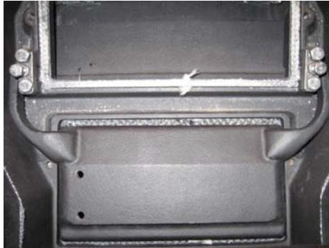
7. When installing the  $\frac{1}{4}$ "-20x 1" bolt in the center of each retainer, pull the bypass door upward so that it is pressed against the under side of the retainers. With the door held in this position tighten the middle bolt until it just touches the door hinges. Now you may release the door. Tighten the bolts one full revolution using the bolt code on the bolt head for easy positioning reference. Tighten the lock nut to keep the bolts in that position.
