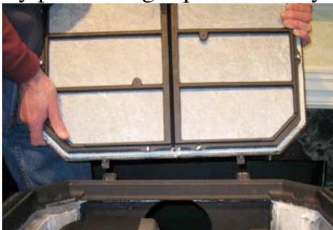
3. If you have not already done so, remove the two transport bolts that hold the combustor assembly in place using  $\frac{1}{2}$ " wrench or socket. (These bolts do not need to be reinstalled as they are for transport only). Remove the combustor and frame assembly from the stove.
