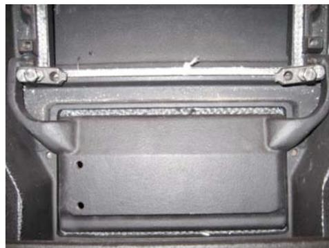
6. Place the new bypass cover into position. Apply anti seize compound to the bolt threads. Swivel the retainers back into position, and secure them with the bolts provided.
