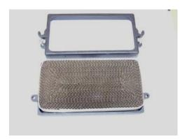
8. Vacuum any fly ash from the combustor scoop and screen. Return the combustor assembly to the stove. The hooks in the top of the combustor frame should point toward the back of the stove. Be sure it is seated properly.
