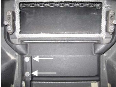
4. Install the new lift guide with the supplied bolts. Apply anti seize compound to the threads of the bolts.
