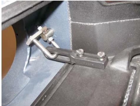
5. Push the U-bolt through the new lift guide. Be sure it is installed in the proper direction. Now push the U-bolt back through the bypass shaft and fasten with the nuts.
