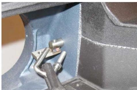
3. Remove the (2) bolts that attach the lift guide to the bypass cover with a ½” socket.
