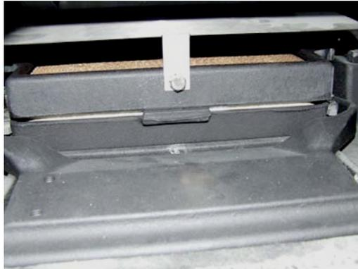
4. If you have not already done so, use a 1/2" wrench to remove the shipping bolts that hold the combustor assembly in place. These bolts are only necessary when the stove is being transported and do not need to be replaced.
