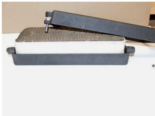
9. Return the combustor assembly to the stove. Be sure it is seated properly. The “hooks” for the shipping bolts should point toward the back of the stove.
