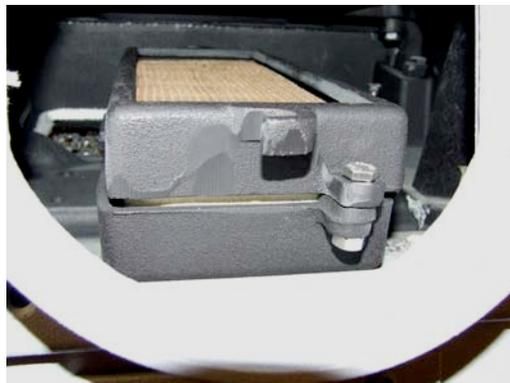
6. Once the assembly has been removed from the stove, use a 7/16" socket and wrench to loosen the bolts that hold the two halves of the combustor frame together. Separate the two halves and remove the ceramic combustor. Remove any residual gasket material from the frame with a putty knife.
