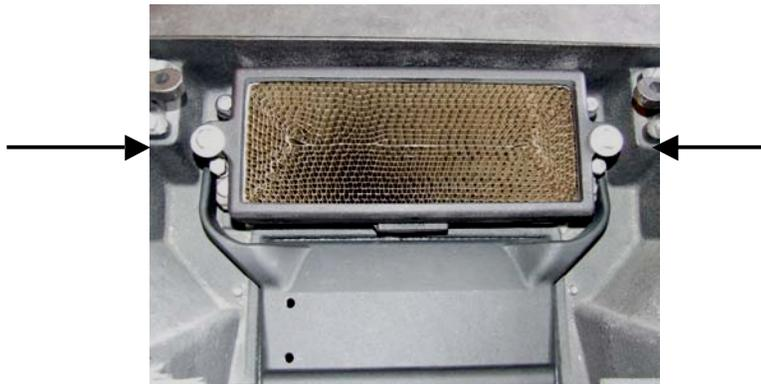
5. The catalytic combustor is housed in a two piece cast iron frame. It will be necessary to rotate the combustor assembly 90 degrees to remove it from the stove.
