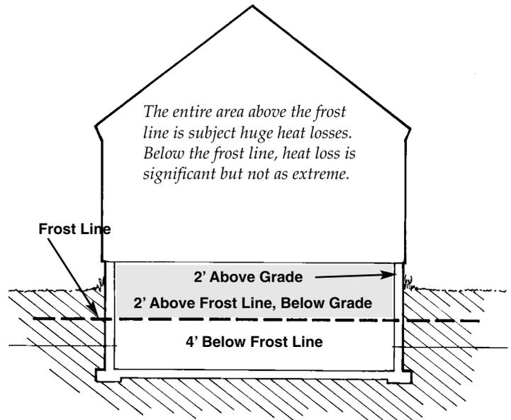
*Temperatures below the frost line are relatively stable at 50°. Heat loss is rapid right down to the frost line.*
