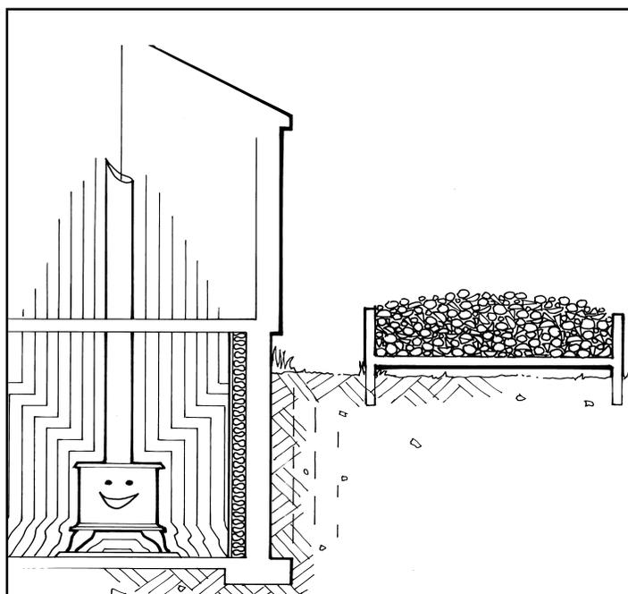
*Insulating your basement walls to R-12 will reduce wood consumption by as much as 16 times in addition to allowing more of your hard won heat to move up into the living areas.*
