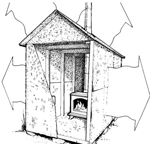
*The heat loss from an uninsulated basement is similar to heat loss from a shed built with 1/2" particleboard walls (R-1.31) and no insulation. You are heating the great outdoors.*
